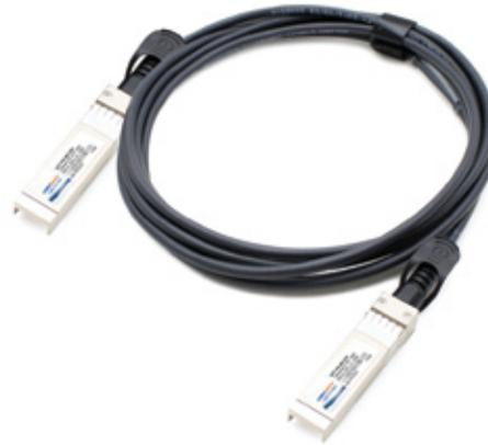
Typically, DAC cables longer than 5 meters are active and draw power from each end, but this may vary from vendor to vendor. Active cables cost three times more than passive cables on average. SFP+ DAC is a popular choice for 10G Ethernet. It reaches up to 10 meters, has low latency and lower cost.
