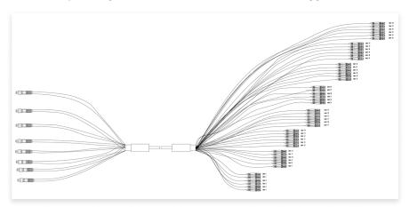
The connection between the Cisco blade and CBX's Port Replication™ Modules is made with fiber optic trunking assemblies, utilizing pre-engineered staggers. The trunking assemblies dress perfectly into the Cisco blade.
