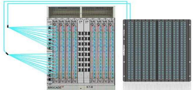
The X7FC64-64 64G blade is connected to the Port Replication module within the 10U modular patch panel.
