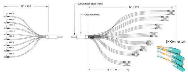
The connection between the blade and module is made with fiber optic assemblies. Utilizing pre-engineered stagers, the assemblies dress perfectly into the blade.
